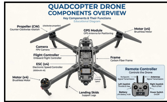
Fig 2.2: Quadcopter drone and its components
